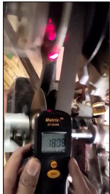
Image 9 CVT DATA COLLECTION WITH RPM SENSOR AND VALIDATION WITH TACHOMETER
